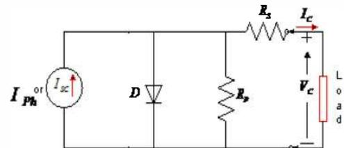
Fig.2. Single diode model of PV source.
