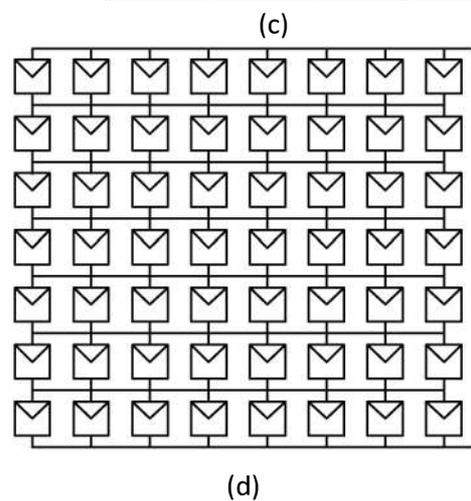
Fig.3 Photovoltaic Array for a) Series-Parallel b) Bridge-Linked c) Honey-Comb d) Total Cross Tied Configurations.
