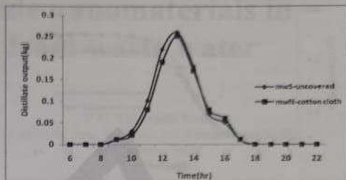
Fig 5. Variation of distillate output through south facing cover on the two consecutive days
