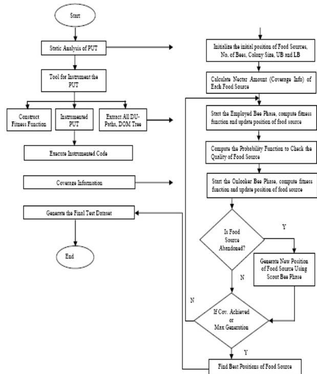
**Figure 4.** Proposed ABC based Test Data Generation framework.
