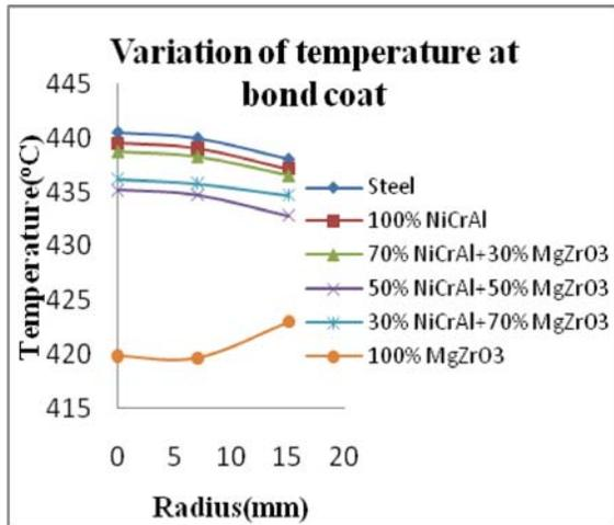
Fig. 3. Variation of temperature at Bond Coat
