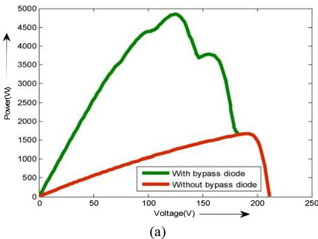
Fig.6.Power-Voltage Characteristics of photovoltaic Array with and without bypass diode for shading pattern P1 a) Series-Parallel b) Bridge-Linked c) Honey-Comb d) Total Cross Tied Configurations.
