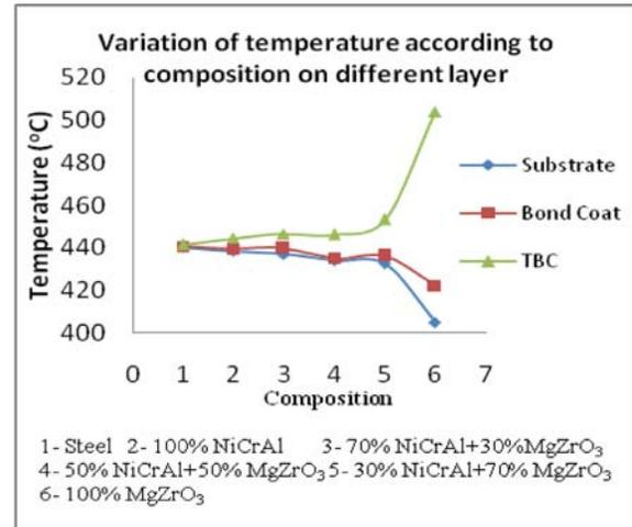
Fig. 4. Variation of temperature according to..Composition on different layer
