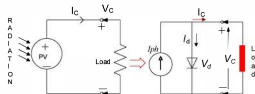
Fig.1. PV cell and its simple equivalent circuit
