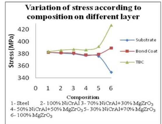
Fig. 10. Variation of stress according to composition .on different layer
