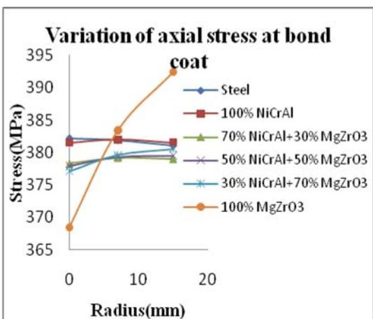
Fig. 8. Variation of axial stress at bond coat
