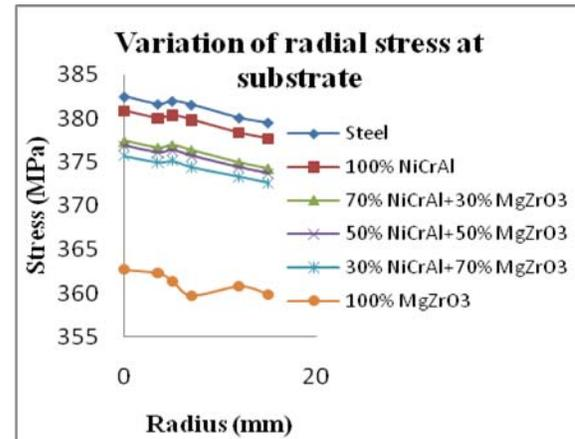
Fig. 5. Variation of radial stress at substrate
