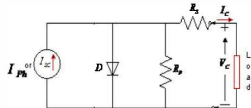
Fig.2. Single diode model of PV source.
