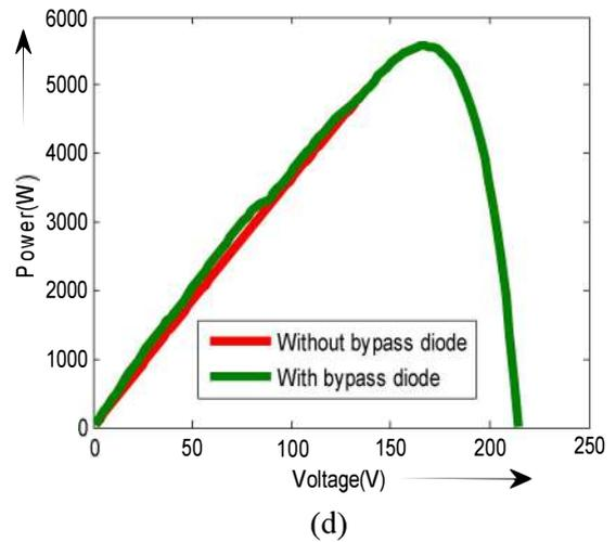
Fig.8.Power-Voltage Characteristics of photovoltaic Array for with andwithout bypass diode for shading pattern P2 a) Series-Parallel b) Bridge-Linked c) Honey-Comb d) Total Cross Tied Configurations.
