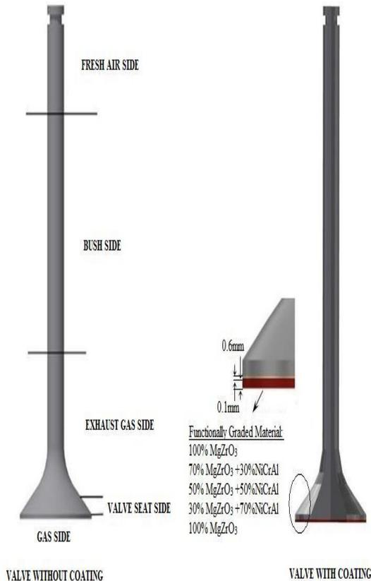
Fig. 1. Valve diagram without and with coating
