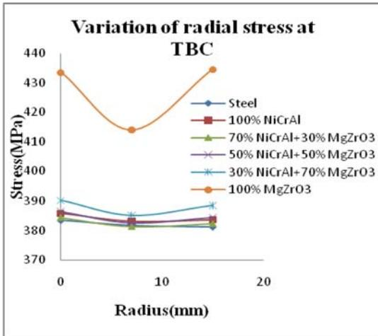
Fig. 6. Variation of radial stress at TBC
